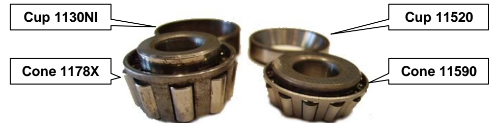
Origineel (OLD) en vervangend lager (NEW)
